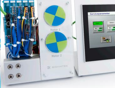
We applied the modularity of out automation complete solution to the SSK 002 starter kit: It consists of the basic control unit TSY 021 in combination with an HMI and motion expansion. You can also order the units individually based on requirements.
